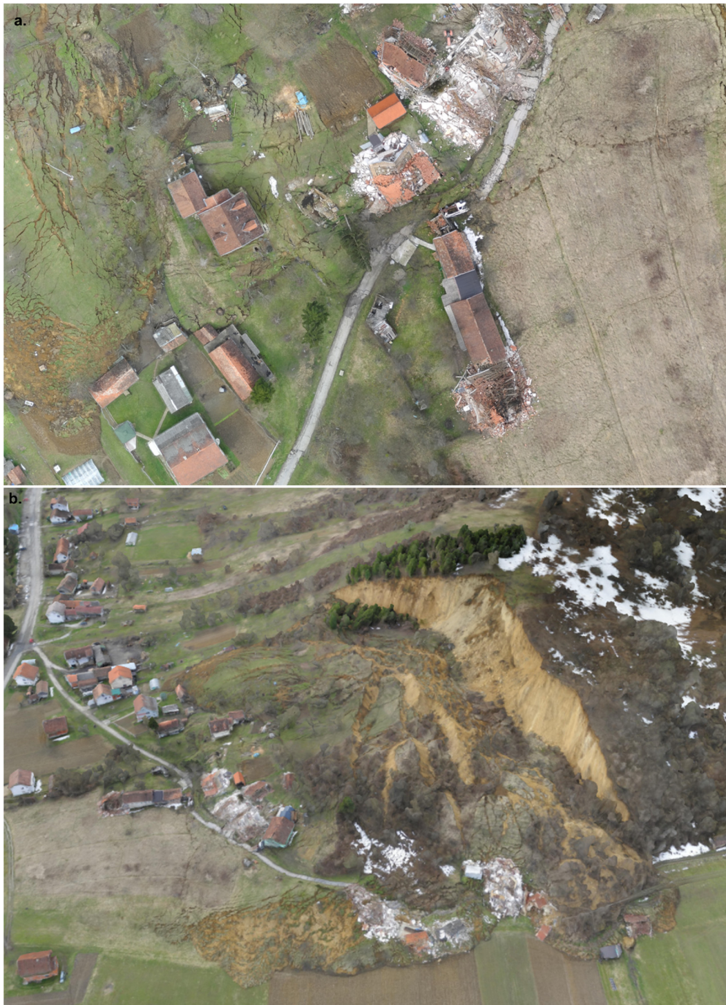
Figure 6. Hrvatska Kostajnica landslide area on 14 March 2018 (day after the event)—UAV data collected, analysed and developed by CGS: (a) detailed orthophoto data; and (b) 3D landslide area spatial model.
