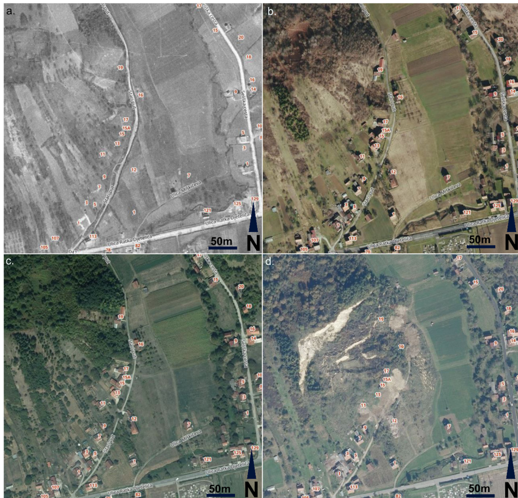
Figure 5. Hrvatska Kostajnica landslide area orthophotos from National Geodetic Administration of Croatia (NGA): (a) from 1968—historical data; (b) from 2016—pre-failure data; (c) from 2018—(recent) pre-failure data; and (d) from 2020—post-failure data.
