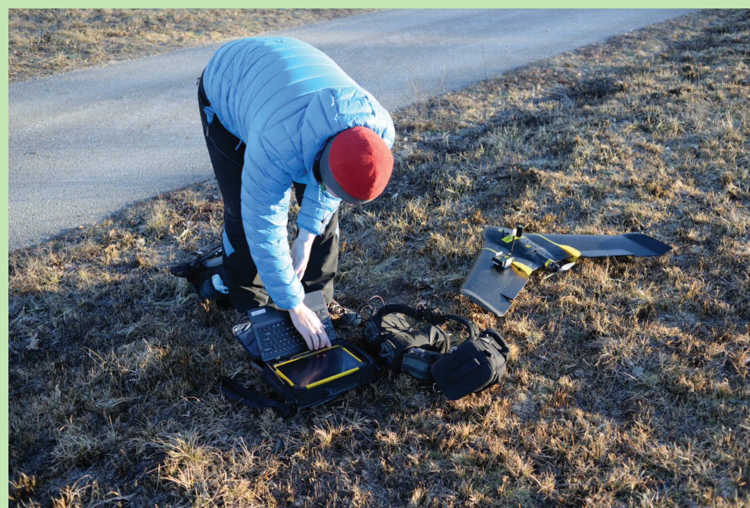
Fig. 4 A geologist operating e-Bee plus UAV used for creating orthophoto image and DSM (Digital Surface Model) of the Pićan area.
