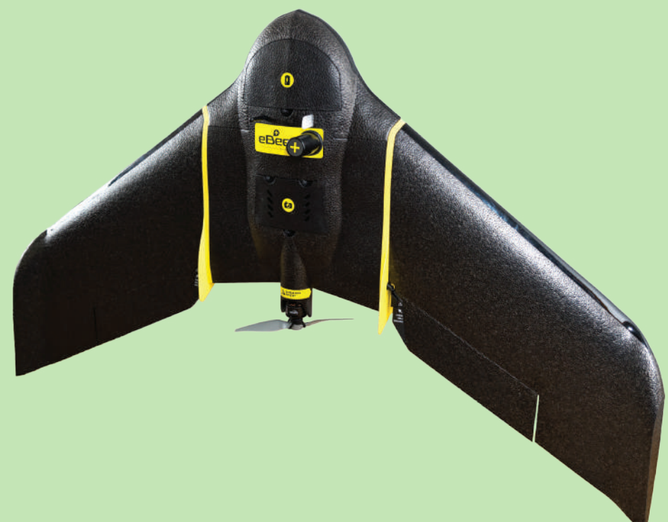
Fig. 4 A geologist operating e-Bee plus UAV used for creating orthophoto image and DSM (Digital Surface Model) of the Pićan area.
