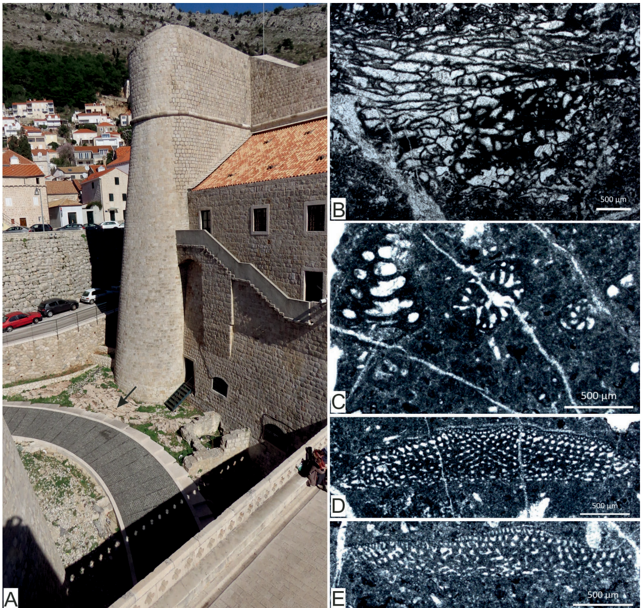
Fig. 7. A) Outcrop of massive yellowish-grey limestone in the basement of the Revelin Fortress (black arrow). B) Photomicrograph of a typical Lithocodium-Bacinella biogenic structure. C) Photomicrograph of Praechrysalidina infracretacea and Voloshinoides murgensis . D–E) Photomicrographs of low-conical orbitolinid foraminifera, the most probably Palorbitolina lenticularis .
