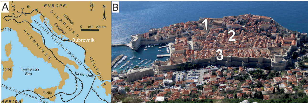
Fig. 1. A) Overview map of the central–northern Mediterranean showing the main orogenic fronts of the indicated fold-and-thrust belts, and the location of Dubrovnik. B) Panoramic view of the Old Town of Dubrovnik from the north (Srd hill): 1 – southern bedrock ridge, 2 – central filled and flattened part, and 3 – northern bedrock ridge (cf. Stanko et al. , 2023; see Fig. 2).
